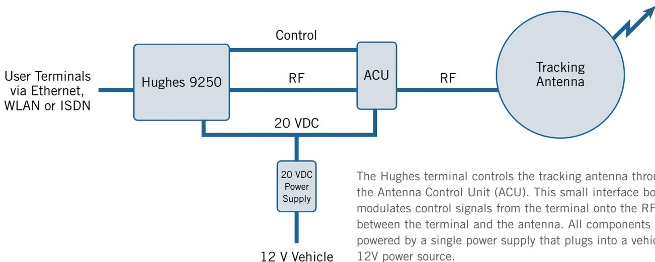
The Hughes terminal controls the tracking antenna through the Antenna Control Unit (ACU). This small interface box modulates control signals from the terminal onto the RF link between the terminal and the antenna. All components are powered by a single power supply that plugs into a vehicular 12V power source.
